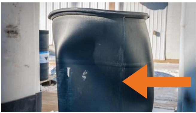
Bulged head or bottom, distorting flange or chime
