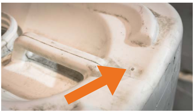
Hole or gash in head, bottom, or body
