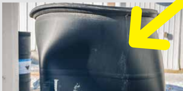
Bulged head or bottom, distorting flange or chime
