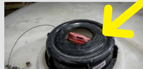
Damage to fittings or deep, sharp crease in body
