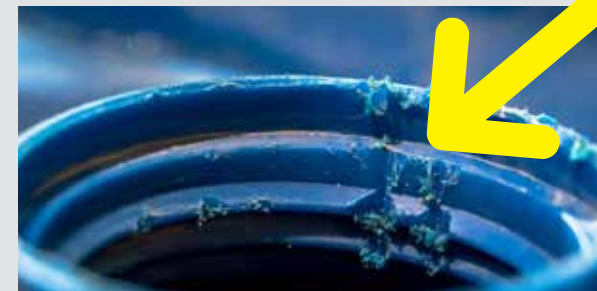
Flange cracked, threads stripped, or weld is broken
